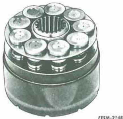
Illust. 2-53. Block assembly removed.
