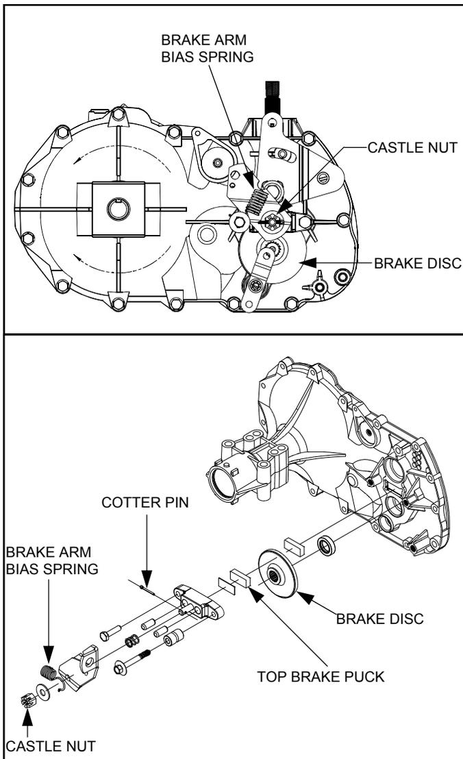
Figure 6. Brake Components
