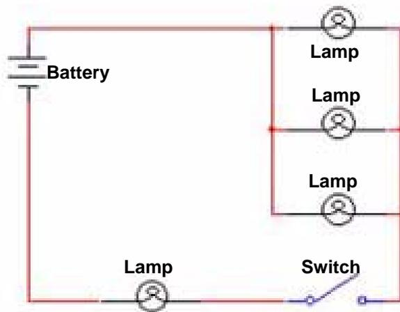
Series/parallel circuits have some sections wired in series and some in parallel. See Figure 7.50.
